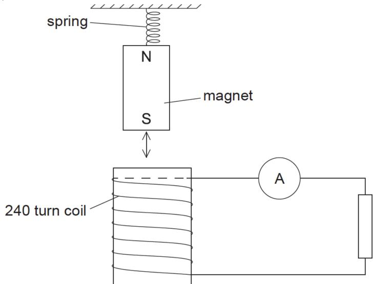
The magnet is displaced vertically and released from its highest position at time *t*=0. Which graph shows the variation with time *t* of the current *l* in the resistor?
