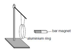
The ring is supported so that it is free to move. The ring is initially at rest. In experiment 1 the magnet is moved towards the ring. In experiment 2 the magnet is moved away from the ring. For each experiment what is the initial direction of motion of the ring?
