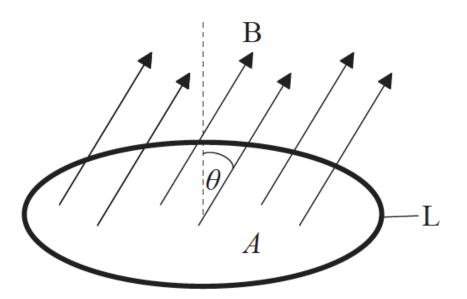
The loop encloses an area A and the field is directed at an angle  $\theta$  to the normal to the plane of the loop. The strength of B is increasing at a uniform rate R. What is the emf induced in L?
