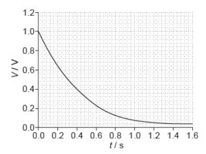
The capacitor is changed to one of value 2C and the resistor is changed to one of value 2R. Which graph shows the variation with *t* of *V* when the new combination is discharged?
