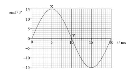
The resistance of the coil is  $5.0 \ \Omega$ . Which of the following is the average power dissipated in the loop?
