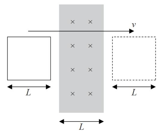
From the instant that the coil enters the field until the instant that the coil leaves the field, which of the following best describes the direction of the current induced in the coil?
