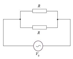
The resistance of each resistor is R and the peak voltage of the ac supply is  $V_0$ . Which of the following is the average power dissipated in the circuit?
