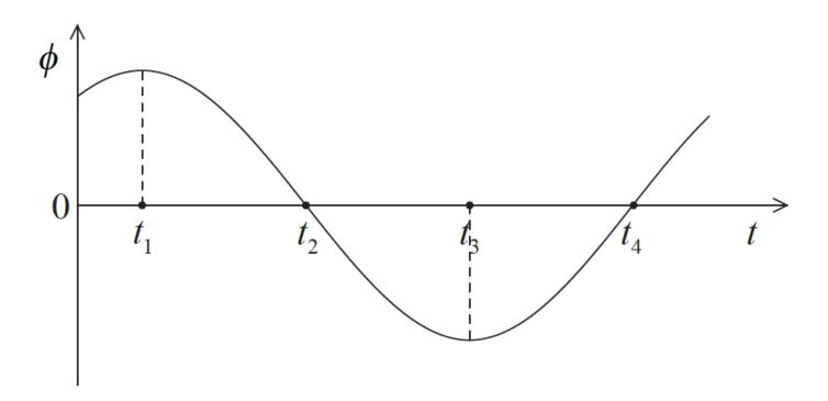
The magnitude of the emf induced across the ends of the coil is maximum at time(s)
