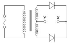
Which graph shows the variation with time of the potential difference V<sub>XY</sub> between X and Y?
