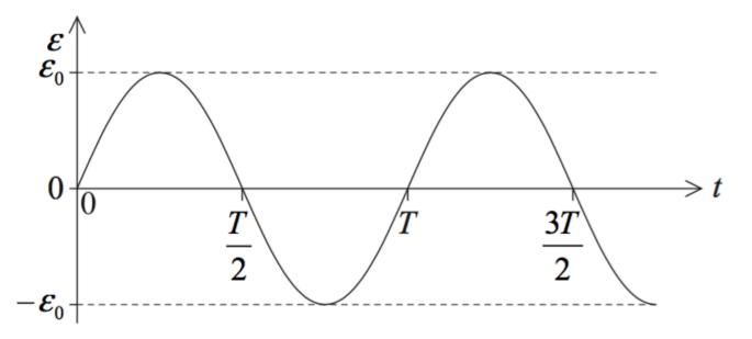
Which of the following correctly gives the rms value of the emf and the frequency of rotation of the coil?
